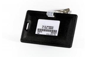
These active RIFD tags are programmed to operate at a 2-second beacon rate. Tag cases are impact resistant, splash resistant and temperature stable. Read ranges up to 1,000 feet can be obtained with optional antenna configurations. The standard tag operates with a very low duty cycle for a long battery life of greater than 3 years (typical) at a 2-second beacon rate.
