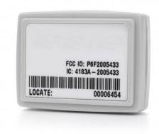
These active tags can be customized to support a broad range of integrated sensors to monitor tag status. Motion activated tags can be programmed to operate at 2 beacon rates: slow when the tag is stationary and faster when the motion sensor is activated, which provides immediate notification when objects are moving. Tamper switches can be installed to trigger an alert if a tag is removed, and panic buttons can be added for personnel and security applications.
