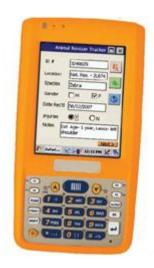
Rugged Handheld Mobile Computer with HF RFID Reader
