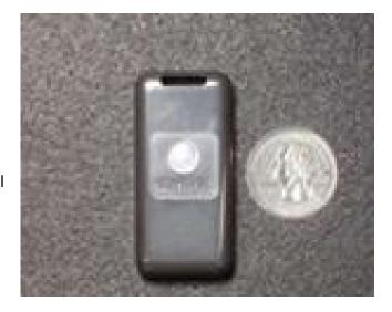
Typically, the tag remains in sleep mode until it receives a wake-up command from an active reader or field generator. If the command is intended for this tag, then the tag will awaken and transmit its ID and other information to an assigned system reader. The tag can also be configured to automatically wake up at predefined intervals, transmit its information to the system, the go back to sleep to conserve battery life.
